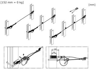
Add 300 kg pretension to the cable system. [134 mm = 300 kg]
