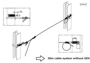
Add pretension to the cable system with the chain crank. [134 mm = 300 kg] Tighten the hex nuts on the loose cable end to the end of the threaded bolt.
