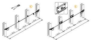
C) longer cable systems with fixed intermediate bracket, compressed every 15m on both sides recommended system length max. 300m
