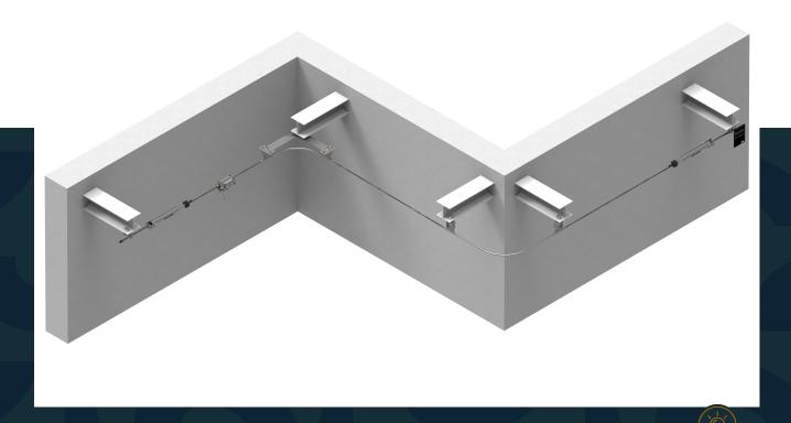
The new passable AIO-GLEIT-22 slider is available from the end of May. Not only does it combine the functions of the existing sliders (curve-compatible and suitable for straight runs), but it can also be mounted and removed at any position in the system. The optimised roller geometry ensures free-running movement in the system. It is delivered in a practical carrying bag.
